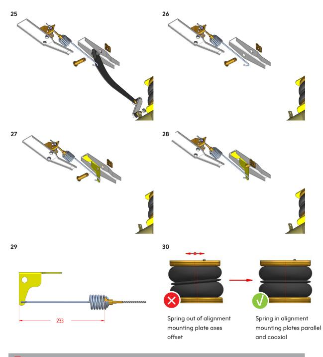
**CAUTION!** - Before fully tightening the bolts that secure the air spring to the upper and lower brackets, set the vehicle at ride height (spring height approximately 13..14 cm) and ensure that the springs are correctly aligned.
