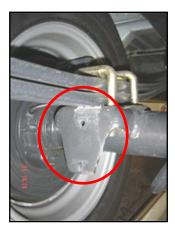
3. Reattach the stabilizer bar to the axle via the mounting brackets, at the same time attaching the lower brackets of the suspension kit. The original bolts may be used. Finger tighten only at this stage.
