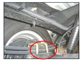
2. Remove the two bolts from the stabilizer bar mounting bracket on each side of the axle
