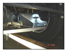
5. Temporarily remove the nuts from the M12 U-bolt that straddles the axis at each end. Pass the bolt through the holes in the lower bracket extension and then reattach the nuts in order to secure the bracket against the axle. Finger tighten only at this stage.
